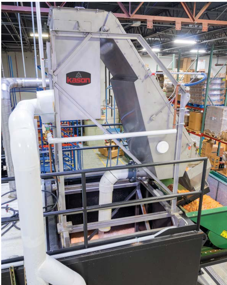
Wastewater is Pumped onto the Dewatering Sieve which Separates Solids at High Rates Without the Use of Power.
